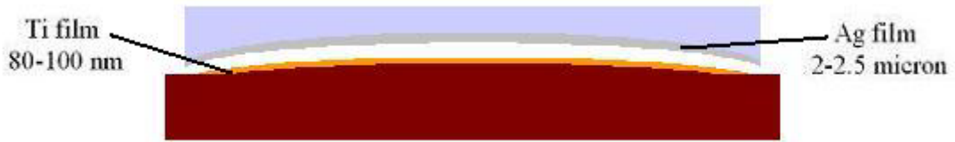
FIGURE 5. Sandwich in Operating Position. Gap is Created Using Mirrored Diodes.
