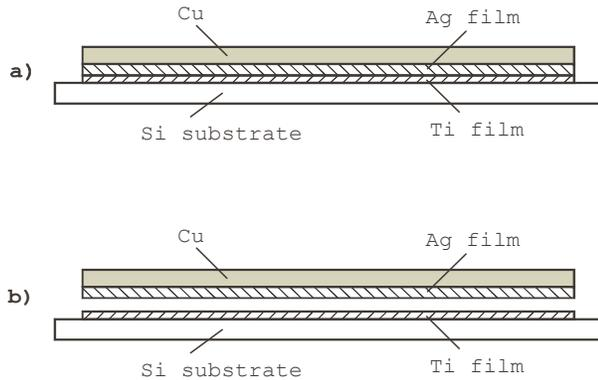
**Figure 1.** a) Si/Ti/Ag/Cu sandwich, b) Opened sandwich comprising Si/Ti and Cu/Ag electrodes having conformal surfaces.
