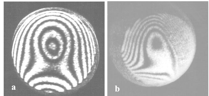
**Figure 2.** Interferograms of two electrodes, a) Si/Ti and b) Cu/Ag. Distance between the rings: 317 nm. Diameter of the Cu/Ag electrode: 28 mm.
