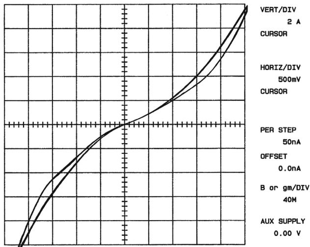
**Figure 3.** I-V characteristic of the sample after opening and adjusting the distance between the electrodes. Hysteresis loop is due to large capacitance between the electrodes.
